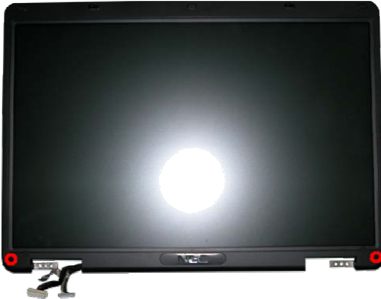
Fig. 25 Screws on the LCD Module
